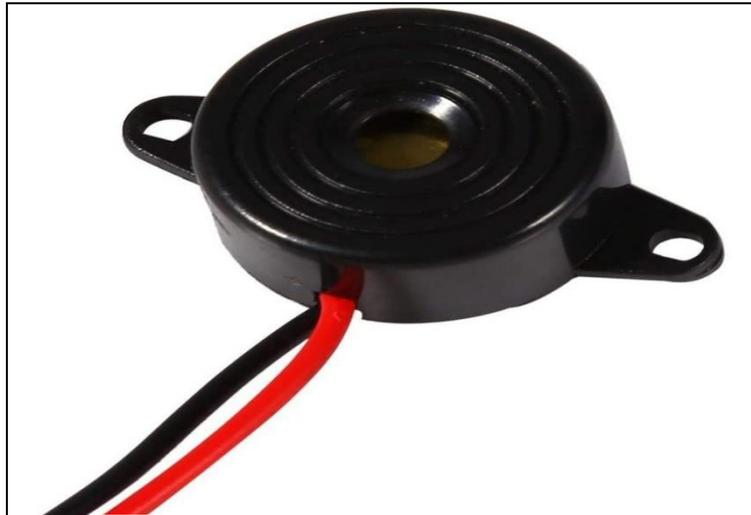
*Gambar 4. 4 Buzzer / Sirine*
