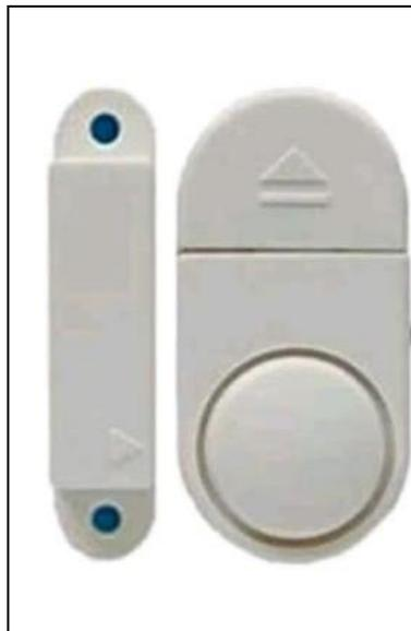
***Gambar 4. 2 Sensor magnetik***
